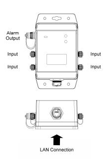
This logger can be used with a CAB-3246 Tinytag Current/Millivolt/Count Input Lead (supplied) or an ACS-9700 2-Pin Plug.
