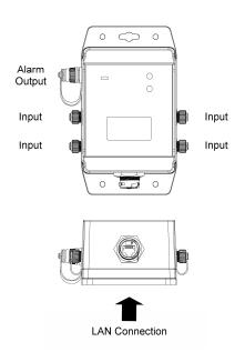
This logger can be used with a CAB-3239 Tinytag Voltage/XP Input Lead (supplied) or an ACS-9703 5-Pin Plug.
