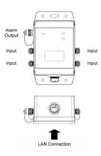
This logger can be used with a CAB-3239 Tinytag Voltage/XP Input Lead (supplied) or an ACS-9703 5-Pin Plug.
