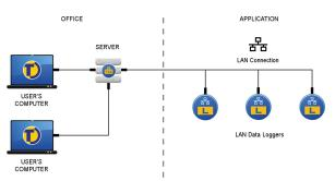
When used as part of a Tinytag Connect system, the logger transmits data to a Windows service that runs the system, called the Connect Gateway. This data is then viewed, and loggers configured, using the Connect version of Tinytag Explorer.
