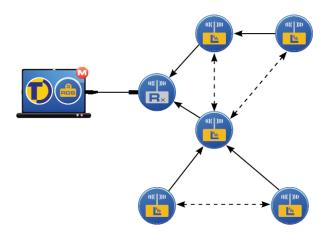
The typical range of the logger on a clear line of sight is 200m.
